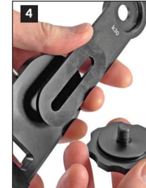
**EN:** Loosen the locking wheel and move the opticsrail (D) to position the hole centrally over the desired lens of your smartphone camera. If your smartphone has multiple lenses - simply align the hole with the lens you want to use. Tighten the locking wheel (C).
