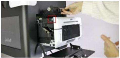
Press the blue button above to access the paper roll, then remove and empty the waste compartment.
