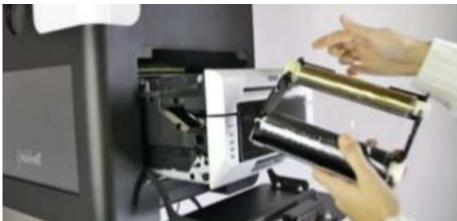
The ribbon with the yellow tip should be on the "handle" side of the holder. Place the holder with the new ink ribbon back into the printer drawer.
