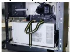
7. (After turning on the device, see 1.3) Reattach the back cover by sliding your fingers into the designated notches. Align the inserts of the back plate with the springs on the device, then push the back plate to securely snap the inserts into the springs.
