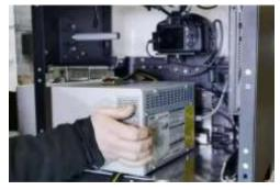
4. Plug the power cable into the printer. This cable is already connected to the power strip. Next, connect the USB cable from the printer, which is already plugged into the tablet.
