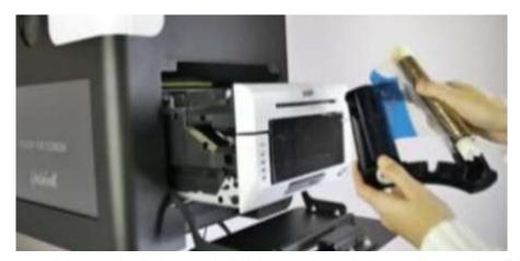
2. Attach the new ribbon to the holder and slightly turn the cylinders to tighten the ribbon.
