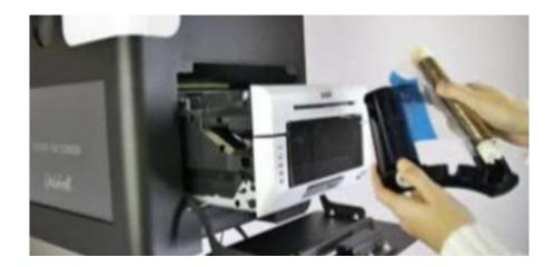
2. Attach the new ribbon to the holder and slightly turn the cylinders to tighten the ribbon.
