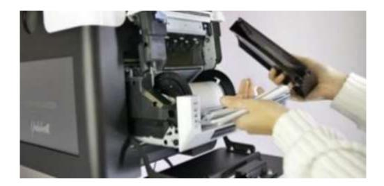
3. Turn the paper roll to remove it from the printer, then take out the two black cylinders from the used paper roll.
