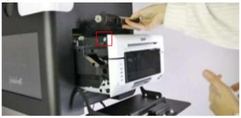
Press the blue button above to access the paper roll and remove and empty the waste compartment.
