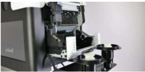
4. The orange "paper" light will start blinking. Insert the two black cylinders on either side of the new roll of paper and place the roll into the printer with the paper facing down.
