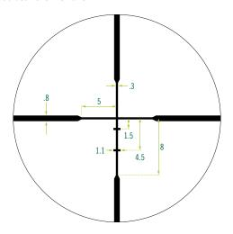
Note: The Muzzleloader BDC reticle is used in Second Focal Plane (SFP) riflescopes. The MOA values are valid at the highest magnification on most models. Please check the Product Manual to ensure what magnification your optic needs to be on
